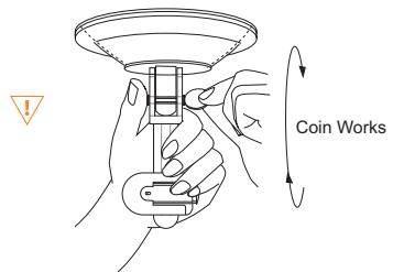
⚠ Warning: Screw to the very end, and check out when loose.
